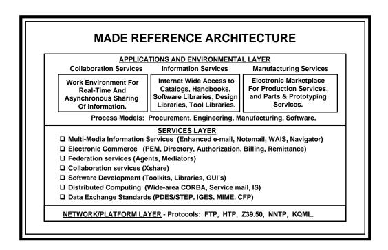
Figure 4. MADE reference architecture.
